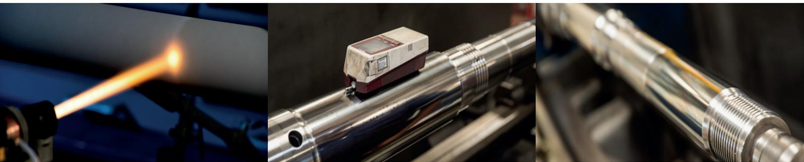
Asco AST coatings are used to combat failures in high wear and corrosive environments to extend the wear life of new and restored compressor rods, piston rods and plungers. Tungsten Carbide and Ceramics are applied, in the range of 0.004" to 0.030", using our latest Thermal Spray systems, in addition we also provide Induction Hardened rods. Seal areas are critical in dry running compressors and subsequently finished to specifications as low as 2 Ra.
